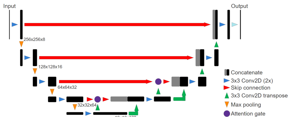
Fig. 3. Schematic of the backbone architecture used in BGRem, adapted from the original attention U-Net (Oktay et al. 2018).
