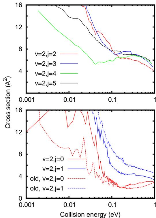
**Fig. 2.** Formation cross section for the reaction  $\text{S}^+(^4\text{S}^o) + \text{H}_2(v, j) \rightarrow \text{SH}^+(^3\Sigma^-) + \text{H}$  for several rotational states and  $v=2$  as a function of collision energy, in logarithmic scale. Results marked “old” (dashed lines) are from Ref. Zanchet et al. (2016).
