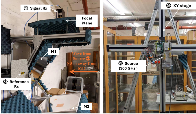
Fig. 14. Laboratory holographic testbed. Left: 1/15 th -scale FYST reflector system (400 mm diameter) with the signal receiver (1) mounted at the focal plane; the reference receiver (2) is placed beside the telescope to provide a phase reference. Right: 300 GHz transmitter source (3), mounted on an XY translation stage (4), is positioned approximately 5 m from the center of the M1 reflector to illuminate the telescope. The telescope beam is measured by raster-scanning the source using the XY stage.
