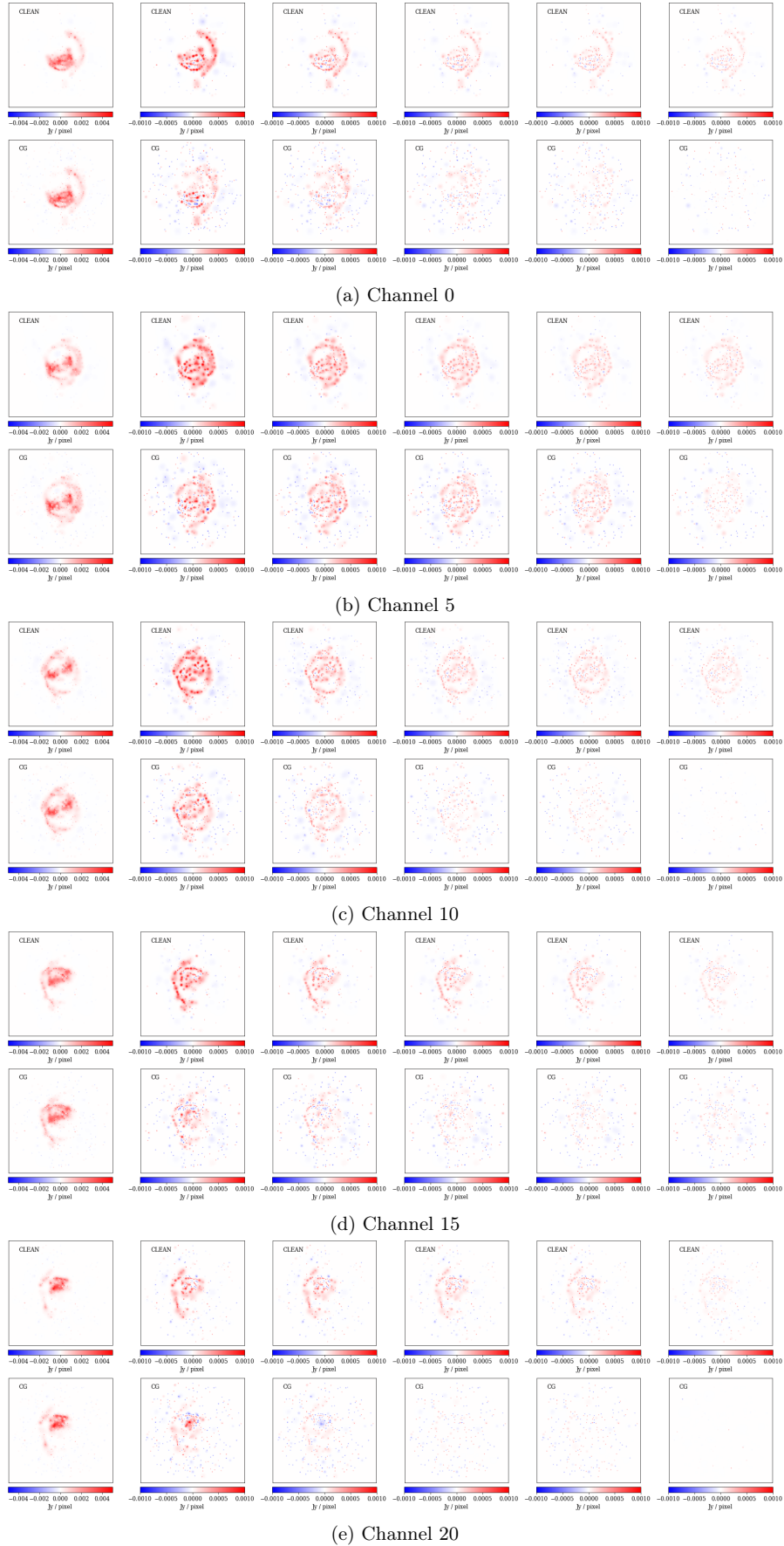
Fig. B.24: Difference between the current model and the final model (after the last major loop iteration) as a function of increasing major loop iterations (from left to right) for NGC 628 with the VLA for CLEAN (top rows in every sub-figure) and CG-CLEAN (bottom row in every sub-figure). The sub-figures show different spectral channels.
