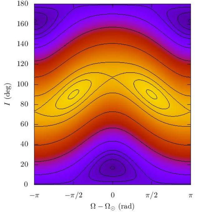
**Fig. 2.** Level curve of the Hamiltonian from Eq. (7). Orbital plane elements will follow the solid lines. One can distinguish four different kinds of equilibrium: one for retrograde orbits, two for polar orbits, and the one we are interested in, for relatively low inclination. The latter gives us  $\Omega = \Omega_\odot$  and both ascending nodes of Iapetus and Titan oscillate around it. Equation (12) and Table 2 give an inclination of the local Laplace plane of Titan around  $0.62^\circ$ .
