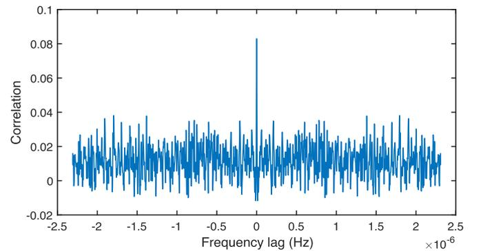
**Fig. C.2.** Cross-correlation between the complete  $g$ -mode model and the power spectrum of the large separation computed on the last 6 yr of GOLF data. The central correlation peak stands also at  $8\sigma$ .
