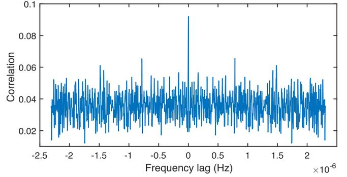
**Fig. 4.** Cross-correlation between a model adding 250  $g$  modes of degree 4 to 168 modes of degree 3, and the large separation power spectrum in the frequency range from 7 to 32  $\mu\text{Hz}$ . The central peak stands at  $7.3\sigma$
