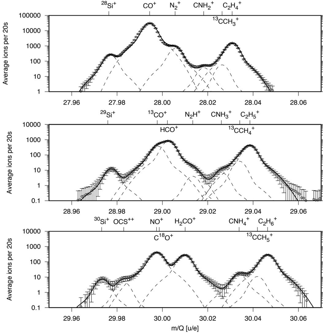
**Fig. 3.** Same as Fig. 1, but co-added over all 288 individual mass spectra and used to derive the reported isotopic ratios of  $^{29}\text{Si}/^{28}\text{Si}$ ,  $^{30}\text{Si}/^{28}\text{Si}$ ,  $^{30}\text{Si}/^{29}\text{Si}$ , and  $^{13}\text{C}/^{12}\text{C}$  in CO,  $\text{C}_2\text{H}_4$ , and  $\text{C}_2\text{H}_5$ .
