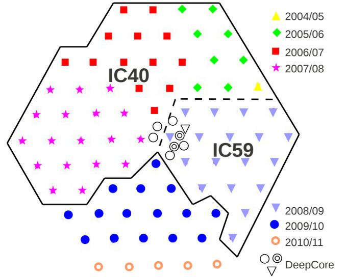
**Fig. 2.** The IceCube detector: The full detector consists of 86 strings with 60 DOMs attached to each string. Different colors/symbols indicate different deployment stages. The solid black line encircles the IC 59 configuration, while the dashed line indicates the smaller IC 40 configuration.
