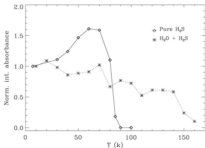
**Fig. 5.** Normalized integrated infrared absorbance of pure H<sub>2</sub>S ice (experiment S3) and H<sub>2</sub>S:H<sub>2</sub>O = 7.5:100 ice (experiment S6, see Table 1) at different temperatures during warm-up.
