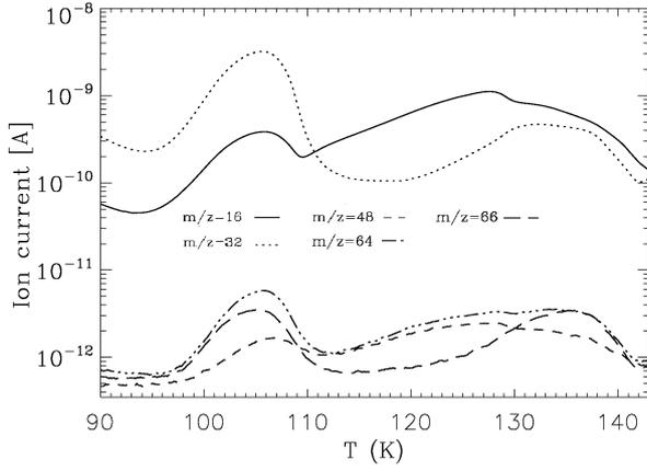
**Fig. 13.** Thermal desorption of UV-irradiated H<sub>2</sub>S:H<sub>2</sub>O = 13:100 in the range of 90–140 K, corresponding to experiment S12 of Table 1. The ion current in Ampere, represented on the  $y$ -scale, corresponds roughly to the partial pressure in mbar.
