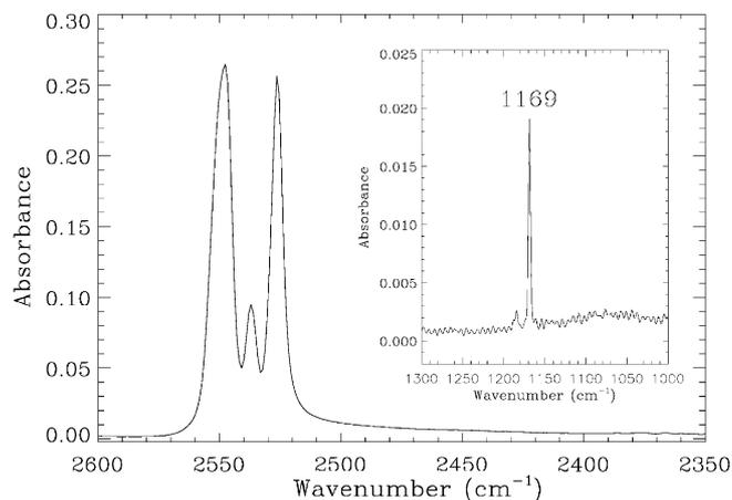
**Fig. 1.** *Top:* infrared spectra of H<sub>2</sub>S ice with 1 cm<sup>-1</sup> spectral resolution at different temperatures during warm-up, corresponding to experiment S2 of Table 1. *Bottom:* infrared spectrum showing the stretching modes of crystalline H<sub>2</sub>S deposited at 70 K. Inlet shows the bending mode absorption.
