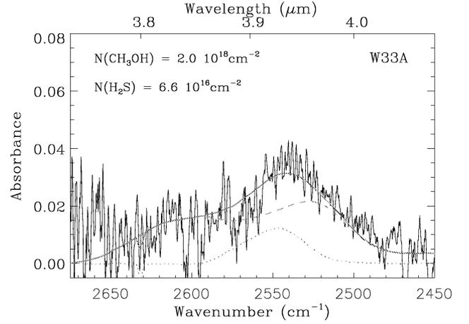
**Fig. 15.** Comparison between our experimental data and the ISO observation of W33A. Dashed line corresponds to the pure CH<sub>3</sub>OH ice spectrum at 20 K, dotted line corresponds to pure H<sub>2</sub>S ice at 20 K, and the continuous line is the addition of both spectra.
