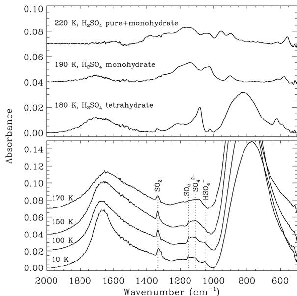
**Fig. 12.** Infrared spectra of the  $\text{H}_2\text{S}:\text{H}_2\text{O} = 13:100$  ice mixture for different temperatures deposited at 8 K, corresponding to experiment S12 of Table 1. The deposition and irradiation was performed simultaneously in this experiment.
