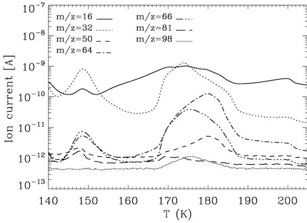
**Fig. 14.** Thermal desorption of UV-irradiated H<sub>2</sub>S:H<sub>2</sub>O = 13:100 in the 140–205 K range, corresponding to experiment S12 of Table 1. The ion current in Ampere, represented on the  $y$ -scale, corresponds roughly to the partial pressure in mbar.
