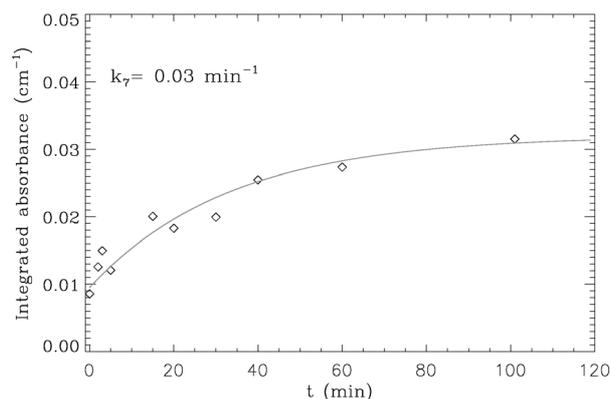
**Fig. 9.** Integrated absorbance values of the 1233 cm<sup>-1</sup> band attributed to H<sub>2</sub>SS ice as a function of UV irradiation time, corresponding to experiment S8, see Table 1. The solid line is a first-order fit using rate constant  $k = 0.03 \text{ min}^{-1}$ , which is probably the value of  $k_7$  from Eq. (14).
