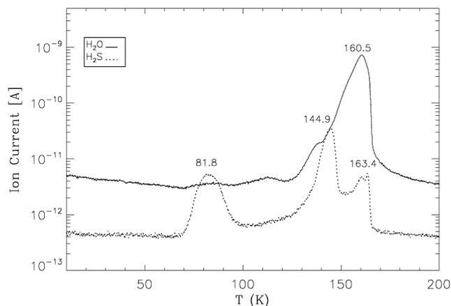
**Fig. 4.** Thermal desorption of the H<sub>2</sub>S:H<sub>2</sub>O = 7.5:100 ice mixture, with a heating rate of 1 K min<sup>-1</sup>, corresponding to experiment S6 of Table 1. The ion current in Ampere, represented on the *y*-scale, corresponds roughly to the partial pressure in mbar.
