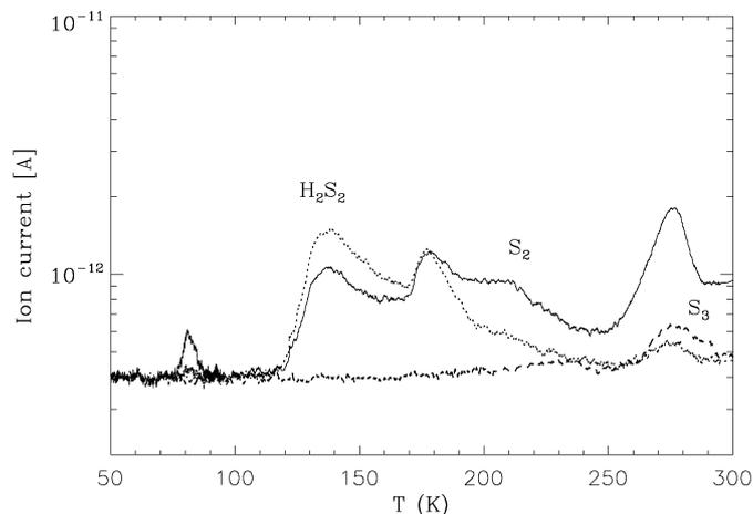
**Fig. 10.** Thermal desorption of UV-irradiated  $\text{H}_2\text{S}$  ice, corresponding to experiment S8 of Table 1. Spectra correspond to  $m/z = 66$  (dotted trace),  $m/z = 64$  (solid trace),  $m/z = 96$  (dashed trace), the molecular ion masses of the  $\text{H}_2\text{S}_2$ ,  $\text{S}_2$ , and  $\text{S}_3$  products. The ion current in Ampere, represented on the  $y$ -scale, corresponds roughly to the partial pressure in mbar.
