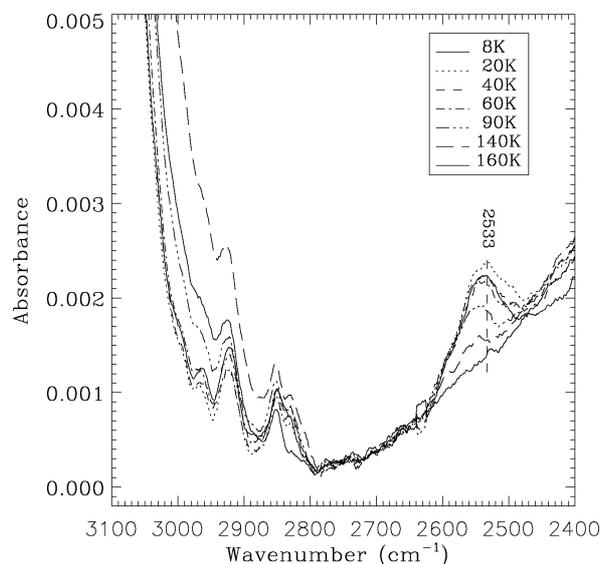
**Fig. 3.** Infrared spectra of the H<sub>2</sub>S:H<sub>2</sub>O = 7.5:100 ice mixture at different temperatures during warm-up, corresponding to experiment S6 of Table 1.
