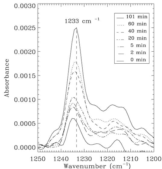
**Fig. 8.** Infrared band around 1233 cm<sup>-1</sup> formed by UV irradiation of H<sub>2</sub>S ice at 7 K, corresponding to experiment S8 of Table 1. Spectra were collected for different irradiation times, see inlet. This band is attributed to H<sub>2</sub>SS based on calculations by Isoniemi et al. (1999).
