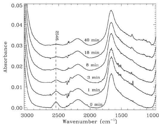
**Fig. 11.** Infrared spectra of the  $\text{H}_2\text{S}:\text{H}_2\text{O} = 4.0:100$  ice mixture at 8 K for different irradiation times, corresponding to experiment S10 of Table 1.
