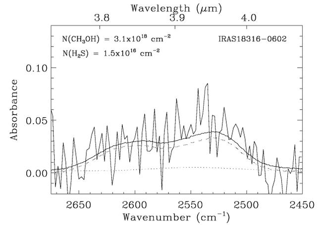
**Fig. 16.** Comparison between our experimental data and the ISO observation of IRAS18316-0602. Dashed line corresponds to the pure CH<sub>3</sub>OH ice spectrum at 20 K, dotted line corresponds to the H<sub>2</sub>S:H<sub>2</sub>O = 13.7:100 ice mixture at 20 K, and continuous line is the addition of both spectra.
