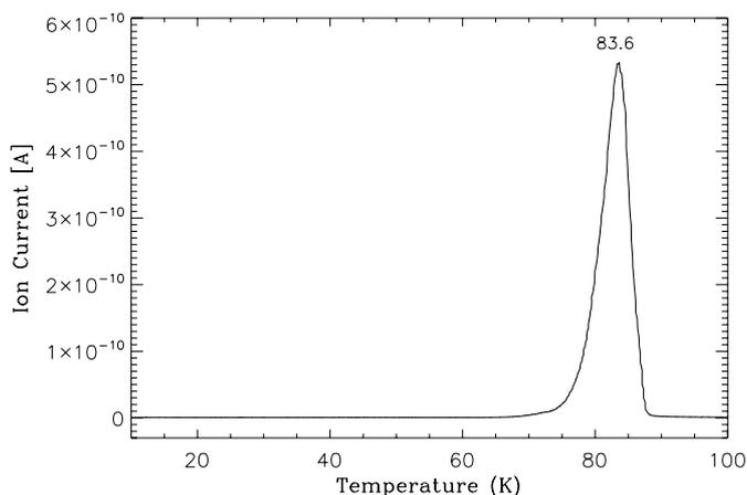
**Fig. 2.** Thermal desorption of pure H<sub>2</sub>S, with a heating rate of 1.0 K min<sup>-1</sup>, corresponding to experiment S4 of Table 1. The ion current in Ampere, represented on the  $y$ -scale, corresponds roughly to the partial pressure in mbar.
