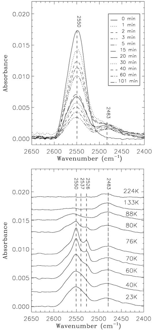
**Fig. 6.** *Top:* infrared spectra of H<sub>2</sub>S ice at 7 K for different irradiation times, corresponding to experiment S8 of Table 1. *Bottom:* for the same experiment, infrared spectra of the irradiated sample collected at different temperatures during warm-up.
