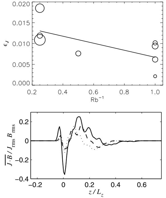
**Fig. 9.** Top: dependence of the total relative current helicity  $\epsilon_J$  on inverse Roberts number. Size of circles codes for value of  $R_m$  (length based). Bottom: dependence of  $\epsilon_J = \overline{\mathbf{J} \cdot \mathbf{B}}/J_{\text{rms}}B_{\text{rms}}$  on  $z$  after saturation for runs B128e (solid,  $Rb^{-1} = 0.25$ ), B128h (dashed,  $Rb^{-1} = 0.5$ ), and B128c (dotted,  $Rb^{-1} = 1$ ).
