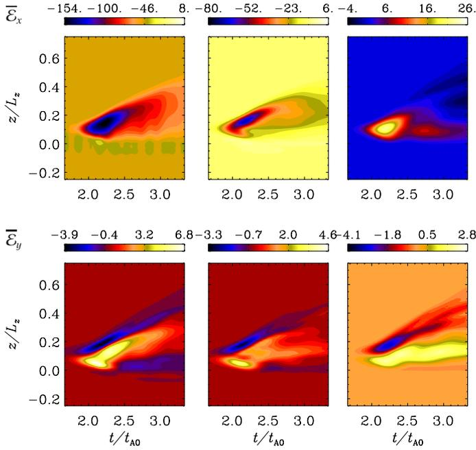
**Fig. 12.** Reconstruction of the mean EMF for the run TF30+ using  $\hat{\alpha}$  and  $\hat{\eta}$  from the test-field method. *Top:*  $\overline{\mathcal{E}}_x(z, t)$ , *bottom:*  $\overline{\mathcal{E}}_y(z, t)$ , both scaled by  $10^{-4}v_{A0}B_0$ . *Left:* directly from  $\mathbf{u} \times \mathbf{b}$ . *Middle:* reconstruction using all contributions  $k' = 0.5, 1, 1.5, \dots, 16$  in (20). *Right:* same as before, but using only the  $k' = 0.5$  contribution.
