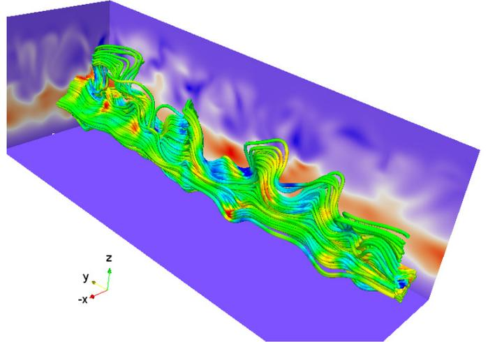
**Fig. 6.** *Left:* volume rendering of the  $B_y = 0.1B_0$  isosurface. *Right:* field lines, colored according to the value of vorticity  $W_y$  for runs B128f (*top*) and B128e (*bottom*) at  $t = 2t_{A0}$  (saturated stage). The contours of  $B_y$  are shown on side walls.
