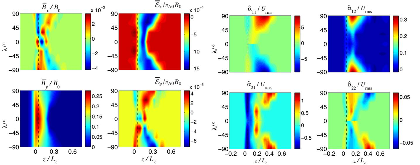
**Fig. 15.**  $\bar{B}_{x,y}(z, \lambda)$ ,  $\bar{E}_{x,y}(z, \lambda)$  averaged between  $t = t^{\text{sat}}$  and  $t^{\text{sat}} + t_{A0}$  from the runs in Table 3 with  $\Omega \neq 0$ . (Initial velocity identical for all latitudes.) Dashed line: initial position of the magnetic layer.
