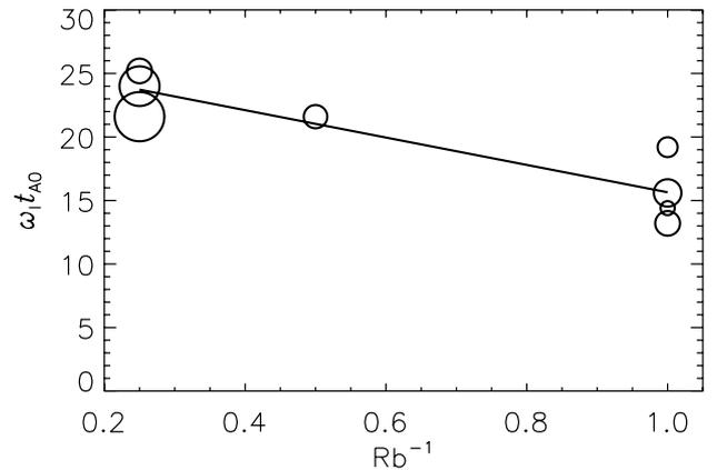
**Fig. 4.** Dependence of growth rate  $\omega_1$  on the inverse Roberts number derived from the runs in Table 2. Solid line: best linear fit. Size of circles corresponds to the value of  $R_m$  (length based, see Table 2).
