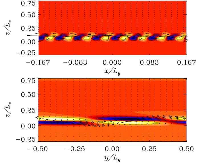
**Fig. 3.** *Top:* velocity components  $U_y$  (in color),  $U_x$  and  $U_z$  (vectors) in the plane  $y = 0$ . *Bottom:*  $U_x$  (in color),  $U_y$  and  $U_z$  (vectors) in the plane  $x = 0$ . Both during the linear evolution phase of the run B128a. The initial condition for  $U$  was set to be harmonic in  $x$  and  $y$  with  $k_x = 8 \times 2\pi/L_x$  and  $k_y = 2\pi/L_y$ .
