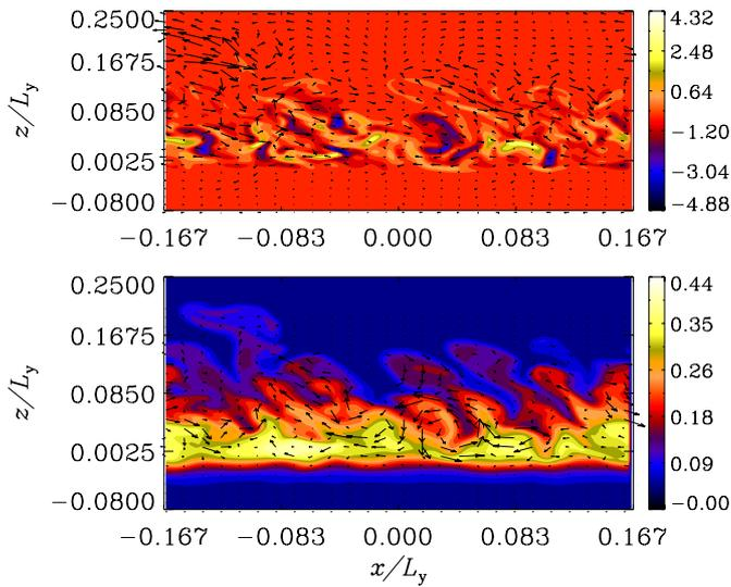
**Fig. 8.** Top: relative current helicity  $\mathbf{J} \cdot \mathbf{B}/J_{\text{rms}}B_{\text{rms}}$  for run B128d at  $t = t^{\text{sat}} \sim 2t_{A0}$ ; arrows:  $v_x$ ,  $v_z$ . Bottom:  $B_y/B_0$  for the same run; arrows:  $B_x$ ,  $B_z$ . Both panels show the plane  $y = 0$ .
