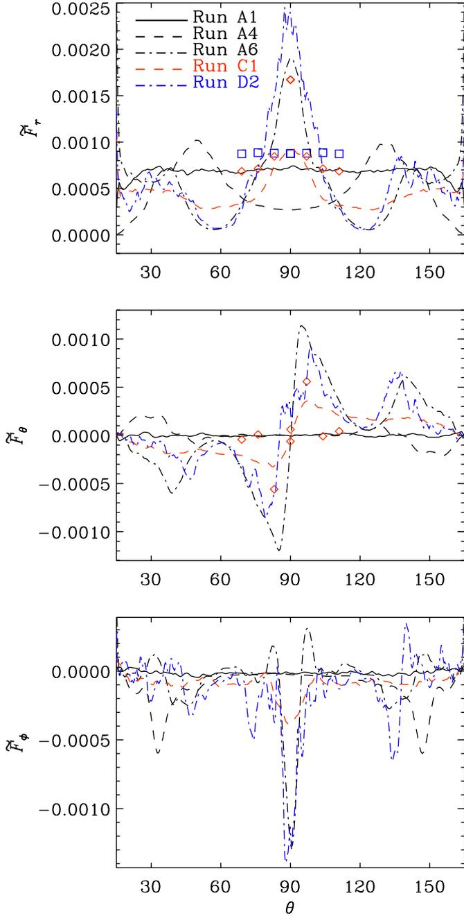
**Fig. 13.** Turbulent heat fluxes  $\bar{F}_r$  (top panel),  $\bar{F}_\theta$  (middle), and  $\bar{F}_\phi$  (bottom) from the runs indicated in the legend in the top panel. The symbols included in the top and middle panels correspond to vertical and latitudinal fluxes from Runs cA1–cA4 (blue squares) and cE1–cE4 (red diamonds) scaled down by a factor of four (see the text for details). The data for Runs C1 and D2 are scaled up by a factor of four.
