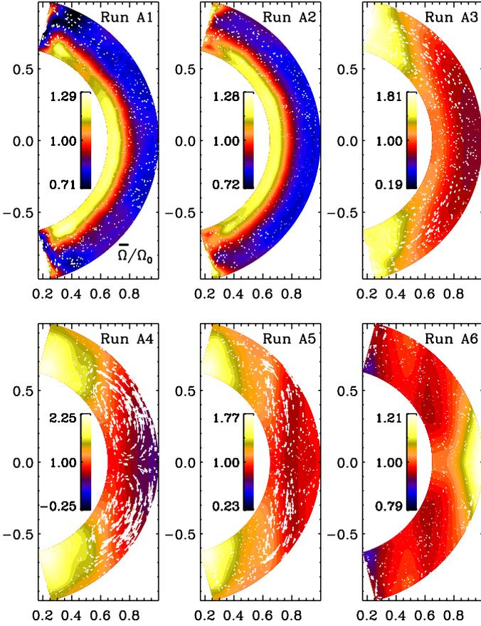
**Fig. 16.** Azimuthally averaged flows from the runs in Set A. The contours show  $\bar{\Omega} = \bar{u}_\theta / (r \sin \theta) + \Omega_0$  and the white arrows denote the meridional circulation.
