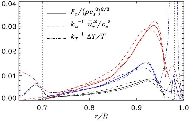
**Fig. 10.** Normalized radial turbulent heat flux raised to the 2/3 power as a function of  $r$  ( $x$ ) (solid lines). The dashed and dot-dashed lines correspond to the squares of the radial velocity and temperature fluctuations scaled with the coefficients  $k_u$  and  $k_T$ , respectively. The upper (red), middle (blue) and lower (black) curves correspond to Runs cA0, cF0 and A0, respectively.
