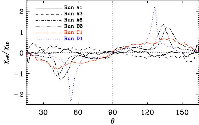
**Fig. 12.** Off-diagonal component  $\chi_{\theta r}$  of the turbulent heat conductivity according to Eq. (43) from Runs A1 (solid line), A3 (dashed), A6 (dot-dashed), B3 (triple-dot-dashed), C1 (red dashed), and D1 (blue dotted).
