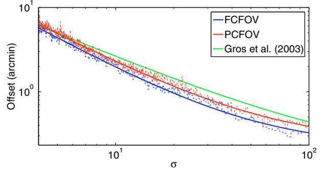
**Fig. 2.** Fits to the OSA 7.0 90% PSLA in FCFOV and PCFOV. In each case, the solid line represents the best fit. We also plot the 90% PSLA estimate of Gros et al. (2003).
