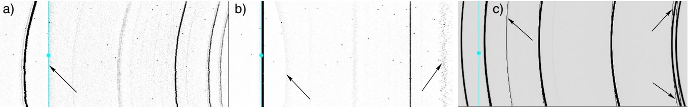
Fig. 4. This figure shows three extracted arc frames of: a) LARR, b) LARR after the dispersion solution was applied, and c) VIRUS-P. Colors are modified to enhance various features. In each panel the vertical line with a disk indicates a preset reference spectrum and wavelength bin. In panel a) the arrow points at the merging point of a shorter (1s; left part) and a longer (10s; right part) exposure. This straight line is curved in panel b) (left arrow). In panel b) the right arrow points at an emission line that was outside the calibration range. In panel c) the left arrow indicates the curved shape of a line in the line mask, after the line geometry has been calculated. The two right arrows indicate a mismatch between the line mask and the data for redder wavelengths. For more details see Sect. 3.3.
