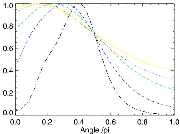
**Fig. 6.** Normalized luminosities for different values of albedo (80% in yellow solid line, 70% in red dotted line, 50% in green dashed line, 20% in blue dashed-dotted line and 0% in black dashed-double-dotted line).
