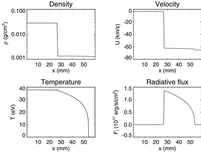
**Fig. 1.** Typical profiles of a 1D radiative shock: density (*upper left*), velocity (*upper right*), radiative and gas temperature (*lower left*), and radiative flux (*lower right*).
