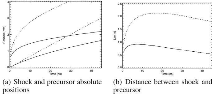
**Fig. 2.** Influence of the dynamics of the piston launching on the shock dynamics. The shock is driven in xenon at 0.2 bar at room temperature. The shock tube is a cylindrical cell with a 0.7 cm diameter and albedo of 40%. The full line refers to the impulsive launching whereas the dotted line refers to a shock driven by a piston at constant velocity of  $65 \text{ km s}^{-1}$  (cf. Sects. 3 and 4).
