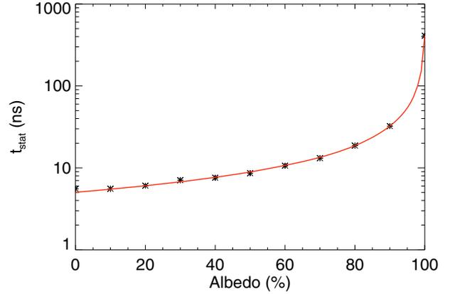
**Fig. 5.** Influence of the albedo upon the time interval to form a stationary radiative shock,  $t_{\text{stat}}$  (points: numerical simulations results, line: fit).
