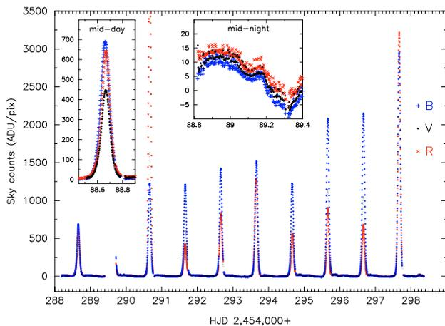
**Fig. 4.** Average background counts in *BVR* for the ten days of our observations. The inserts show an example of the counts during midday (*left*) and midnight (*right*), respectively. *BVR* is indicated with different plot symbols (pluses *B*, dots *V*, crosses *R*).
