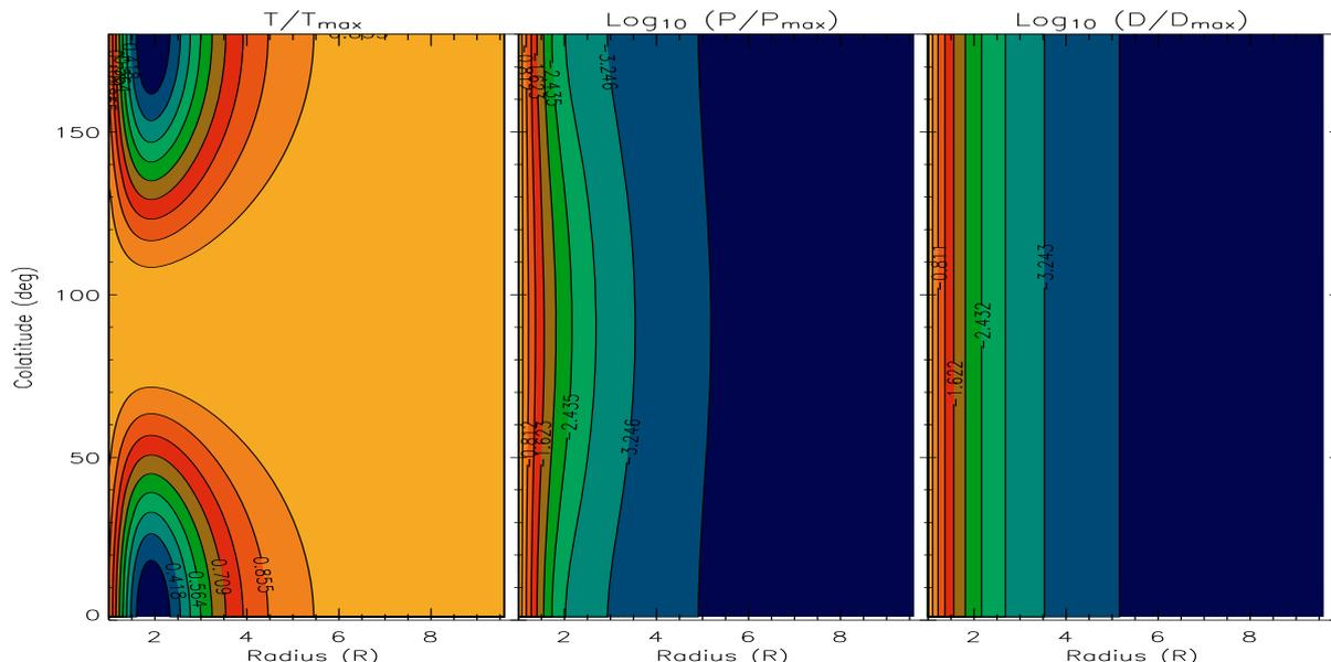
**Fig. 3.** Relative temperature (*left panel*), logarithm of the relative pressure (*middle panel*) and of the relative density (*right panel*) for an illustrative coronal model computed for HD 179949 (see text for details).
