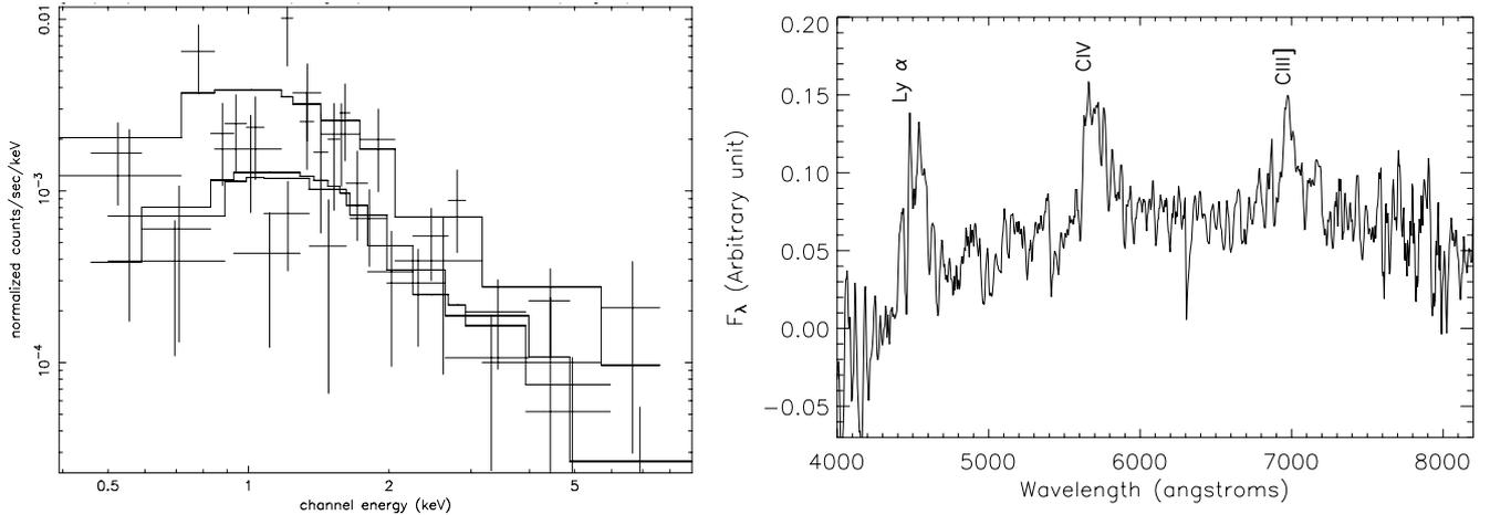
**Fig. 15.** MOS1 MOS2 (the two lower functions) and pn (upper one) X-ray spectra of a source which is showing strong X-ray absorption with  $N_{\text{H}}^{\text{int}} = 4 \times 10^{22} \text{ cm}^{-2}$ . The crosses represent the data points and the solid line represent the folded model simultaneously fitted to the data of the 3 detectors (*left*). The optical counterpart has been identified as a BLAGN lying at a redshift  $z = 2.66$  (*right*). This is source #20 in Table 4.
