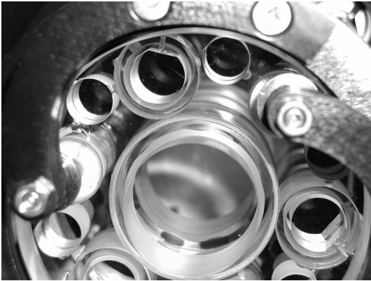
Fig. 13. Close-up of the VUV FPI etalon assembly with the housing removed. Shown are two of the three curved cantilever springs with the piezoelectric stack beneath. In the center are the MgF_2 etalon with the VUV coatings and, hence, clear in the visible. At the top between the two springs are two capacitance bridges and one reference bridge.
