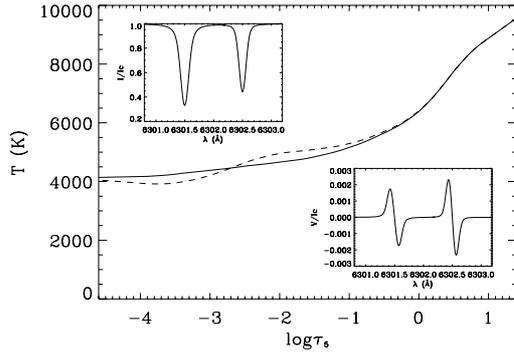
**Fig. 7.** Temperature stratifications for the synthesis of the Stokes vector used for the numerical test. The solid line is the temperature stratification for the non-magnetic component and the dashed line for the magnetic one. The small plots inserted are the Stokes  $I$  and  $V$  profiles synthesized from them (see text for details).
