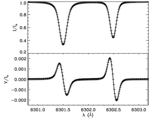
**Fig. 3.** Fits to 1000 G synthetic  $I$  and  $V$  profiles at 630 nm with different model atmospheres having the following fixed field strengths: 100, 300, 500, 700, 900 and 1000 G. Plus signs represent the synthetic profiles and lines are the fits.
