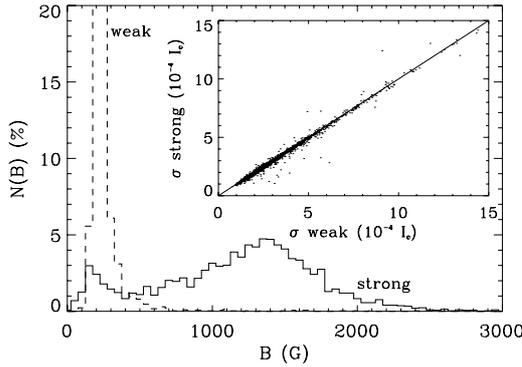
**Fig. 13.** Magnetic field distribution recovered from the observed data using two different inversions, with a strong (solid line) and a weak (dashed line) magnetic field strength initializations. The small plot represents the standard deviation,  $\sigma$ , of the difference between the observed and the fitted Stokes  $V$  profiles. The overplotted continuum line is the diagonal.
