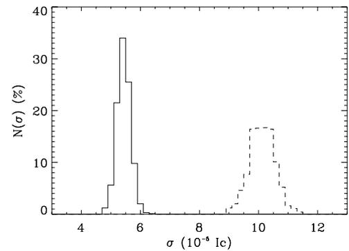
**Fig. 9.** Standard deviations of the difference between the noisy synthetic profiles and their fits. The solid and dashed lines represent the cases with a noise level of  $5 \times 10^{-5} I_c$  and  $10^{-4} I_c$ , respectively. The inversion procedure assumes the same temperature stratification with optical depths and microturbulence for both the magnetic and the non-magnetic components.
