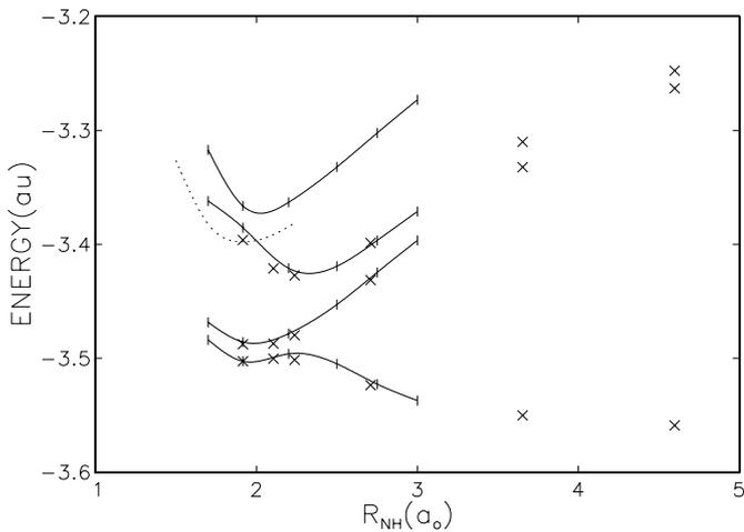
**Fig. 3.** The four lowest adiabatic potential curves of linear HCNH as a function of  $R_{\text{NH}}$ . The dotted line is the ion curve. The tic marks on the curves indicate the points at which calculations were performed. The solid curve is a spline. (The calculated energies have been shifted uniformly by +90 au.) The symbol (x) denotes the calculations of Talbi & Ellinger (1998), shifted vertically to agree with the present results at the ion equilibrium position.
