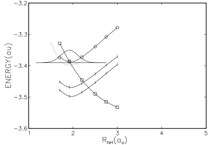
**Fig. 4.** The four diagonal elements of the diabatic Hamiltonian as a function of  $R_{\text{NH}}$ . The dotted line is the ion curve. (The calculated energies have been shifted uniformly by +90 au.) The  $v = 0$  level of the ion and a harmonic oscillator wave function is shown ( $R_{\text{NH}}$  motion only). The symbols (O) and (□) indicate the diabatic curves dominated by the antibonding orbital  $\sigma_{\text{CH}}^*$  and  $\sigma_{\text{NH}^+}^*$ , respectively.
