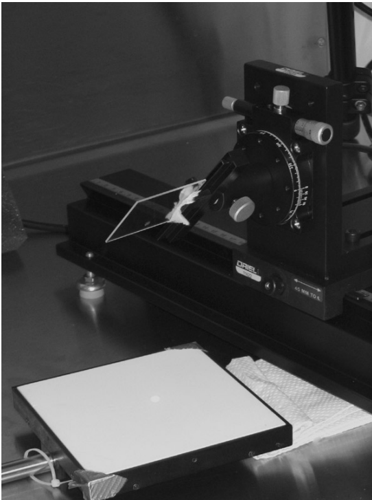
Fig. 2. A detail: the beamsplitter with its holding point and a Spectralon plate.
