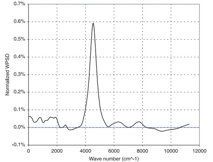
**Fig. 1.** Average wavelets power spectral density (WPSD) of the 464 processed interferograms of NGC 1068. The subtraction of the background noise from the processed fringes' power peak left no residual bias on the final WPSD. The power integration is done between wave numbers 2000 and 8000  $\text{cm}^{-1}$ .
