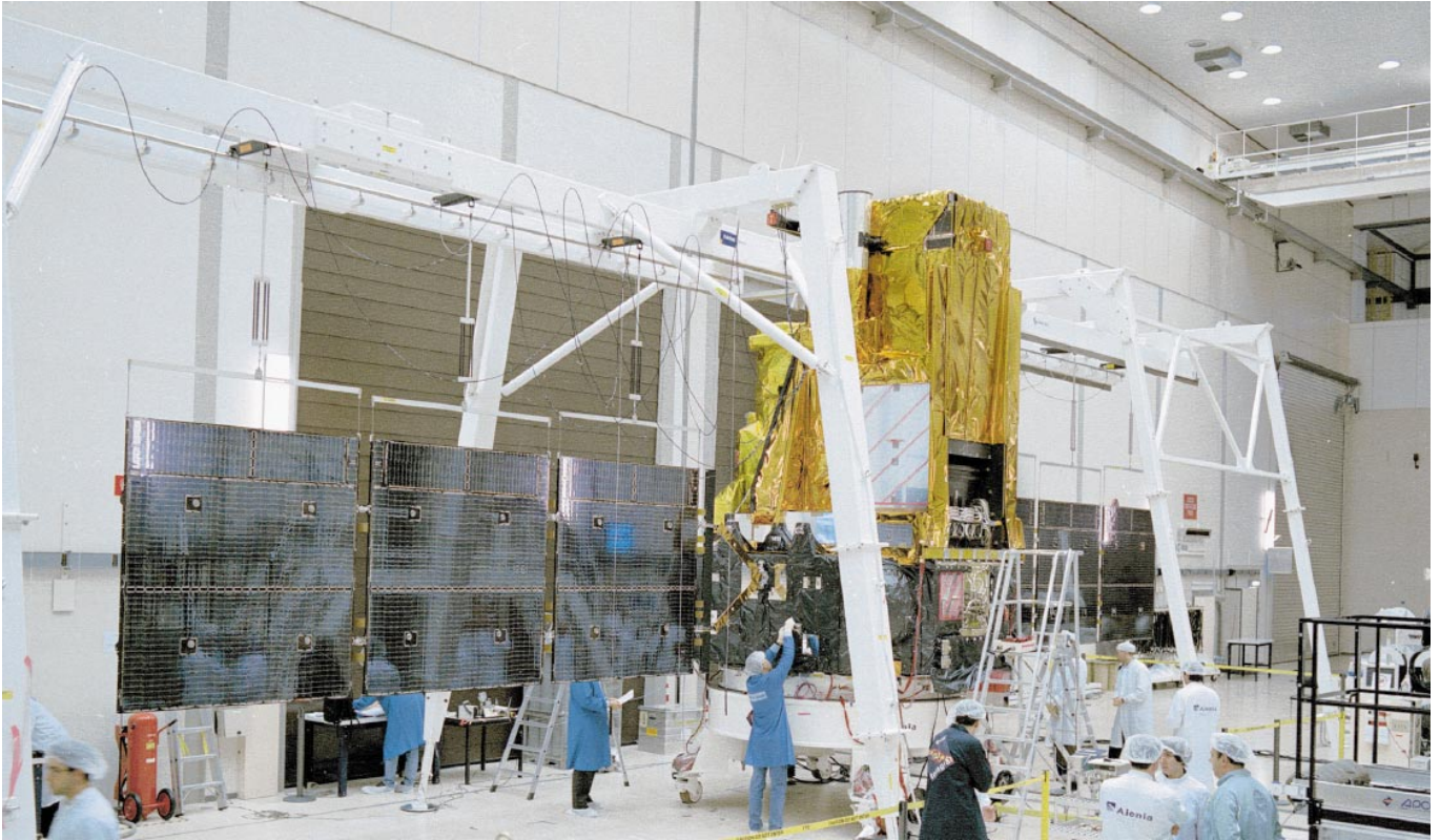
Fig. 1. The INTEGRAL flight model during solar array deployment testing at the ESTEC test facility.
