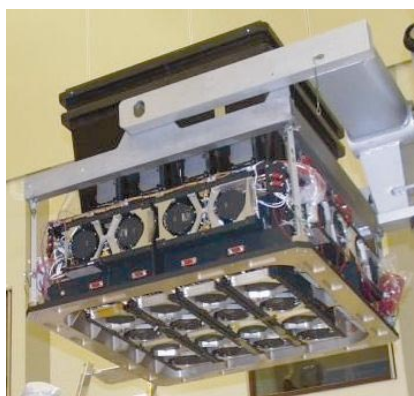
Fig. 2. IBIS showing lateral and rear veto.
