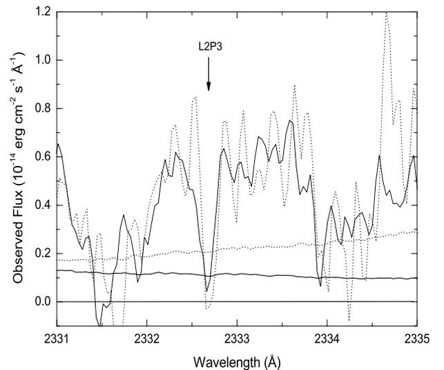
**Fig. 1.** Typical example for a relative wavelength shift between successive orders. The H<sub>2</sub> L2-0 P(3) line shows a difference of  $\Delta\lambda \sim 0.04 \text{ \AA}$  ( $\Delta v \sim 5 \text{ km s}^{-1}$ ). The lines at the bottom indicate the noise level.
