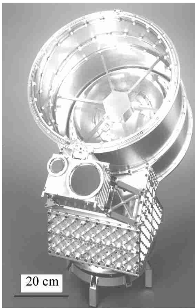
Fig. 1. Cassini Cosmic Dust Analyser flight spare, courtesy of Heidelberg Max-Planck-Institut für Kernphysik. The hollow drum like structure in the top half of the figure is the main body of the instrument. The target is at the bottom of this drum and the ion detector is mounted in the hexagonal assembly suspended in the middle of the drum. Suspended beneath the circular opening of the main detector is a rectangular box with two circles on the front face. This is a high rate dust flux monitor using pvdf impact momentum sensors.
