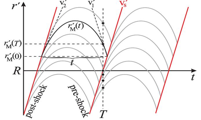
**Fig. 1.** Reconstruction of the radial structure of a shock wave at position  $R$  for time  $T$  (dots) from periodically shocked Lagrangian elements assuming ballistic trajectories (grey lines). Dark grey lines indicate the trajectories of the periodic shock fronts.
