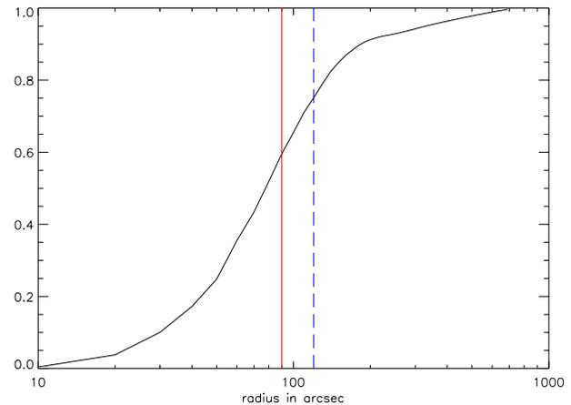
**Fig. 4.** Growth curve of the effective footprint on a logarithmic scale with the location of the radii of circles used for aperture photometry; dotted vertical line: 90 arcsecond for the inner radius; dashed vertical line: 120 arcsecond for the outer radius.
