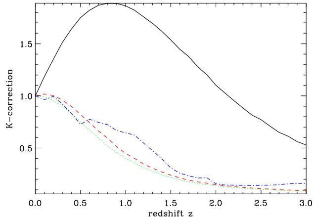
**Fig. 1.** K-corrections at 15 (dot-dashed curve), 60 (dotted curve), 90 (dashed curve) and 170  $\mu\text{m}$  (solid curve) for a LIRG (Dole 2000; Lagache et al. 2001). The wavelengths of cosmological interest are thus around 15  $\mu\text{m}$  and above 150  $\mu\text{m}$  where they benefit from the “negative K-correction effect”, increasing the sensitivity up to redshifts around unity.
