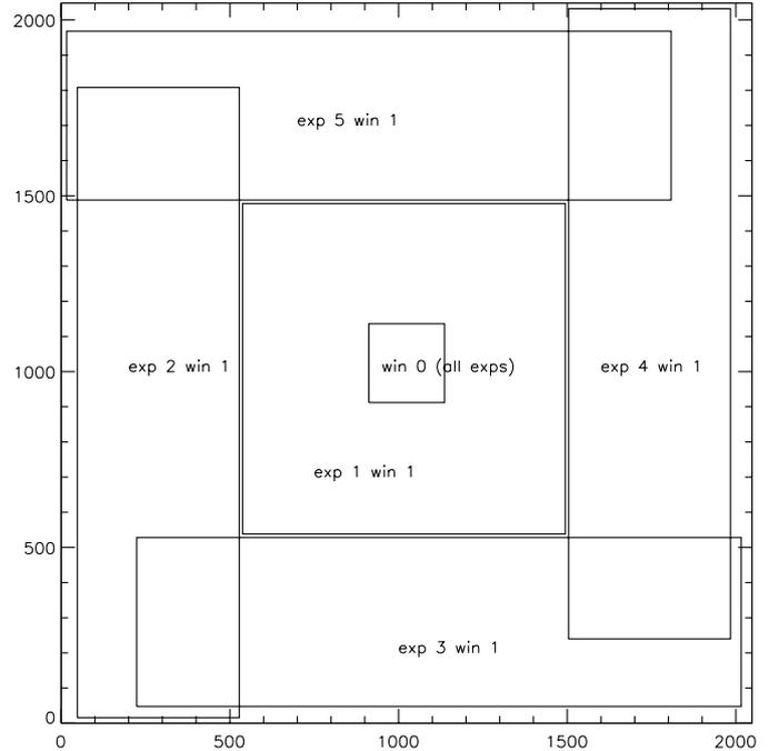
**Fig. 2.** Setup of XMM-OM imaging default mode. There are 5 exposures, each one being made up of two image mode windows: win 0 and win 1. Win 0 is the same for each exposure and is unbinned (0.5 arcsec). Win 1 for each exposure is binned  $2 \times 2$  pixels and the position changes for each exposure. For exposure 1, win 1 is a square containing the central half of the FOV, with win 0 entirely inside it. For the other exposures, win 1 is arranged to fill in the rest of the FOV
