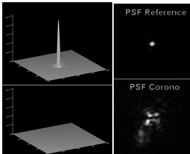
**Fig. 4.** *Top-left:* the 3D representation of the non coronagraphic PSF with a linear intensity scale. *Bottom-left:* the 3D representation of the coronagraphic PSF, normalized to the non-coronagraphic image peak intensity. *Top- and bottom-right:* the corresponding 2D images, but with two different photometric scales, so that the coronagraphic image is visible. The peak-to-peak intensity ratio is  $\sim 1000$ .
