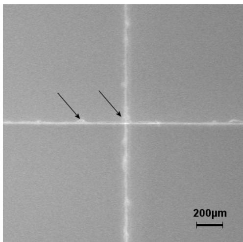
**Fig. 3.** Image of the coronagraphic mask illuminated by a diffuse white light source. Black arrows point toward defects (bubbles) produced by an optical oil used to avoid humidity infiltration. At the cross intersection, a faint defect is affecting the coronagraphic performance by modifying the image intensity distribution (see Fig. 4-bottom right).
