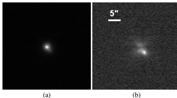
**Fig. 7.** On-sky data of HD 80081. **a)** Without the coronagraph (monitoring camera); **b)** with the coronagraph (science camera). This image was obtained by co-adding 126 frames selected among the 5000 recorded frames, using the selection algorithm described in Sect. 6.2. The companion appears clearly in the coronagraphic image.
