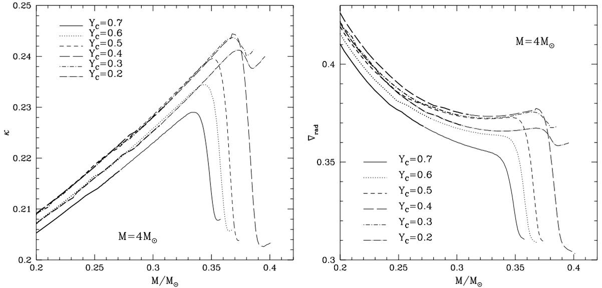
**Fig. 5.** The internal distribution of opacity (*left panel*) and radiative temperature gradient (*right*) within the core of a  $4 M_{\odot}$  model at the same evolutionary stages of Fig. 4. We see that the increase of the opacity coefficient at the border of the core leads eventually to the formation of a local minimum of  $\nabla_{\text{rad}}$ .
