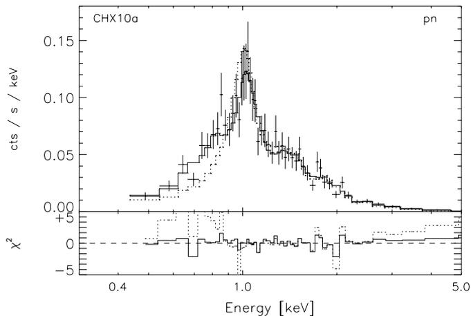
**Fig. 4.** EPIC pn spectrum of CHX 10a overlaid by the 1-T (dotted histogram) and 2-T (solid histogram) bestfit model. The lower panel shows the  $\chi^2$  residuals. Clearly the 1-T model does not adequately describe the data.
