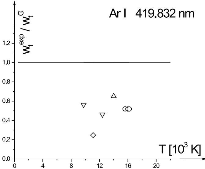
**Fig. 2.** Ratios of the experimental total Stark *FWHM* ( $W_t^{\text{exp}}$ ) to the theoretical ( $W_t^{\text{G}}$ ) predictions (Griem 1974) vs. electron temperature for  $\lambda = 419.832$  nm.  $\circ$ ,  $\diamond$ ,  $\nabla$  and  $\triangle$  represent our experimental data and those from Kusz & Mazur (1996), Bues et al. (1969) and Gericke (1961), respectively.
