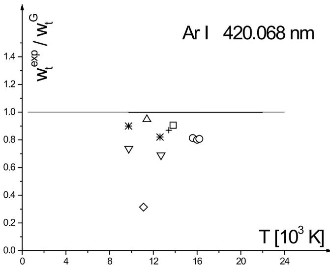
**Fig. 3.** Ratios of the experimental total Stark *FWHM* ( $W_t^{\text{exp}}$ ) to the theoretical ( $W_t^{\text{G}}$ ) predictions (Griem 1974) vs. electron temperature for  $\lambda = 420.068$  nm.  $\circ$ ,  $\square$ ,  $\diamond$ ,  $\nabla$ ,  $\triangle$ ,  $*$  and  $+$  represent our experimental data and those from Chapelle et al. (1967), Kusz & Mazur (1996), Bues et al. (1969), Gericke (1961), Griem (1962) and Musielok (1994), respectively.
