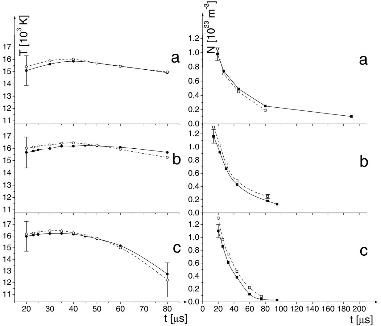
**Fig. 1.** Electron temperature ( $T$ ) and density ( $N$ ) decays. Full lines represent measured data using independent experimental techniques. Dashed lines represent plasma parameters obtained using our line deconvolution procedure in various plasmas (see a, b and c in Table 1). Error bars represent estimated accuracies of the measurements ( $\pm 11\%$  and  $\pm 7\%$  for  $T$  and  $N$ , respectively) and deconvolutions ( $\pm 12\%$ ).
